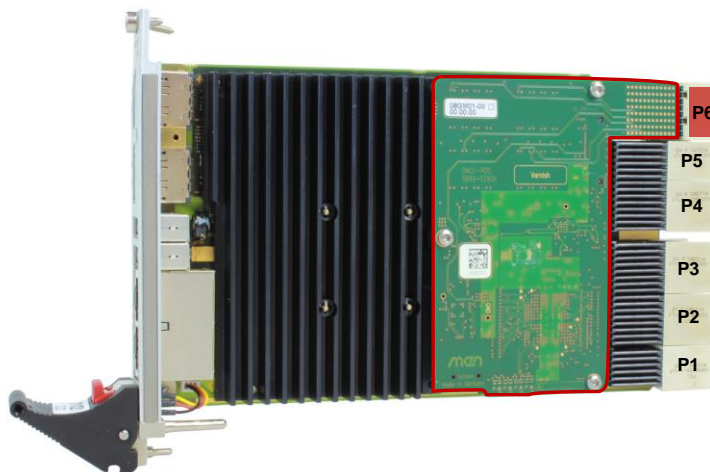
Mezzanine with backplane connector P6 for Ethernet configuration of the system slot CPU
