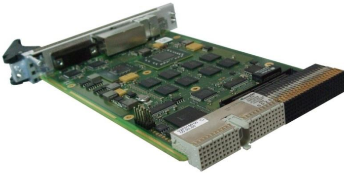
CompactPCI PlusIO CPU card with new J2 connector (shown individually at the right)
