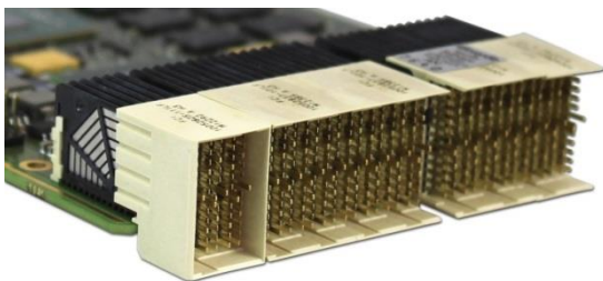
CompactPCI Serial: Compared to CompactPCI the plug and receptacle are swapped
