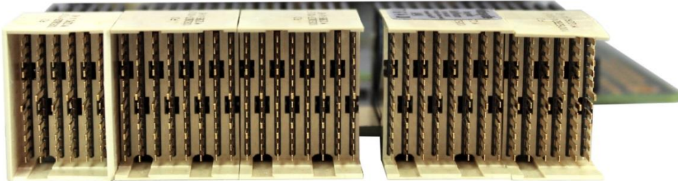
CompactPCI Serial: Row of connectors on a plug-in board
