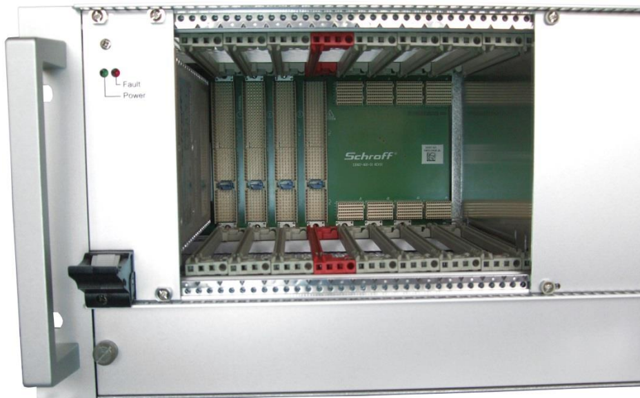
Hybrid backplane in a 19" system
